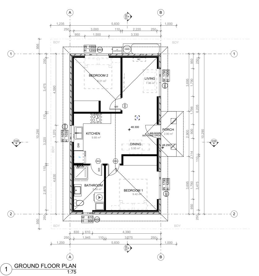
LOCATION OF DOWN PIPE (DP). BUILDER TO CROSS CHECK WITH APPROVED STORMWATER PLAN.
